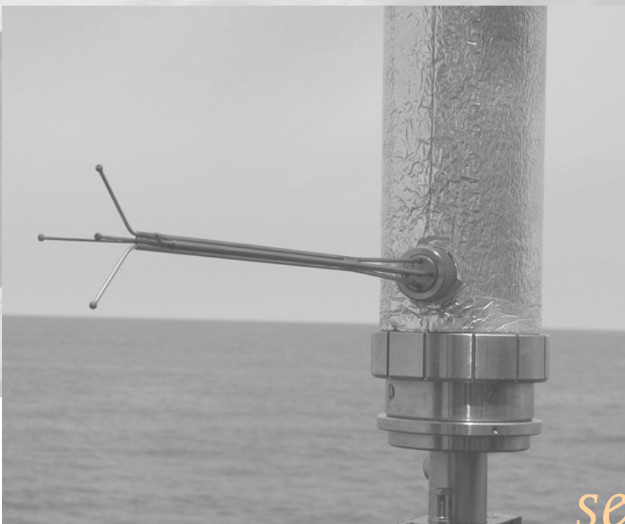
Figure 4. Photograph showing a pressure anemometer (PA). The version of the PA shown here was constructed especially for use on the wave follower. The flow outlet tubes can clearly be seen.
