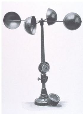
Figure c: The Robinson anemometer. In: The Aims and Methods of Meteorological Work by Cleveland Abbe. In: Maryland Weather Service, Johns Hopkins Press, Baltimore, 1899. Volume I, p. 316. Image ID: wea00920, NOAA's National Weather Service Collection
