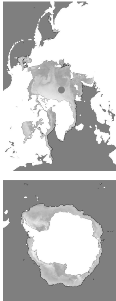
Fig. 4. Arctic and Antarctic sea ice extents for May 15 th 2007 from scatterometer (QSCAT-KNMI) with sea ice GMF noise \text{std}[\sigma^0_{ice}] = 1.5 dB. Background grey scale represents sea ice backscatter strength.
