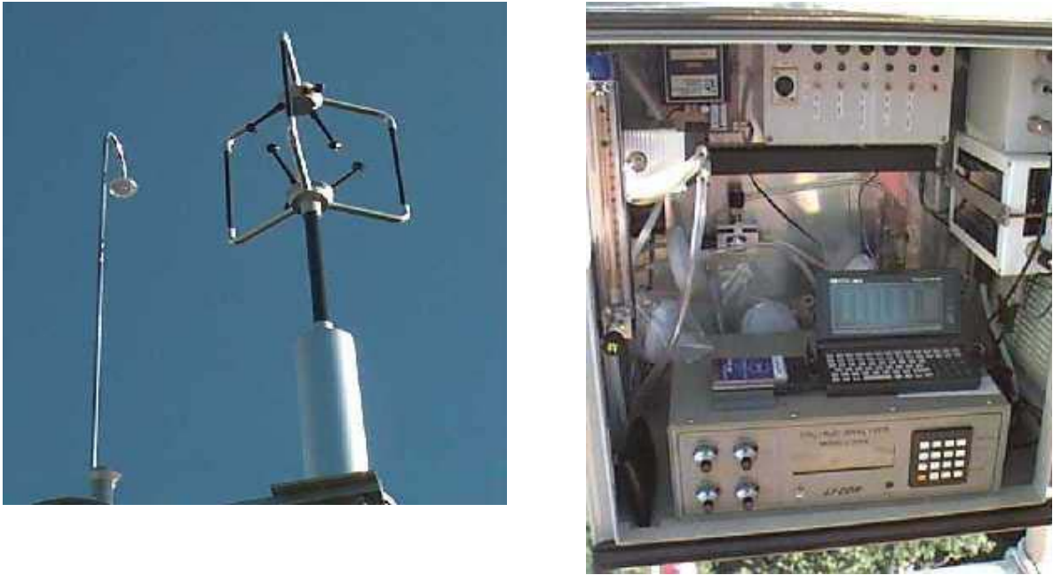
Figure 1. Eddy correlation devices at the Loobos site. Left: Ultrasonic Anemometer and air inlet for CO 2 and H 2 O measurements. Right: gas analyzer. See text and references for further information.
