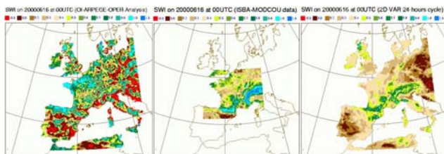
Figure C: Comparison between soil moisture content obtained from an operational OI system using air temperature and humidity (left), a best estimate based on observed precipitation and radiation (center), and a variational technique using the same observations as OI (right) (Balsamo et al., 2002)
